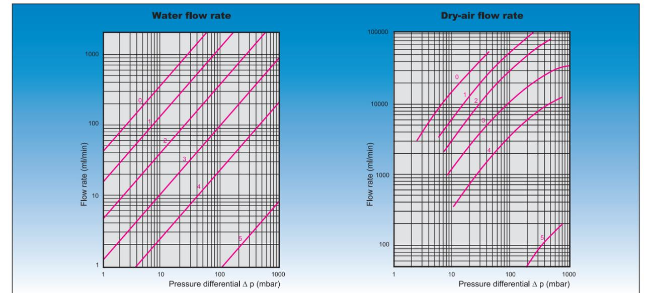
Fig. 1: Water and air flow rate through filter discs of various porosities as a function of pressure differential. For disc diameter 30 mm.
